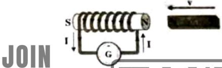
b) When the North Pole of the bar magnet is moving away from the face of the coil it becomes a South face by the induction of current in clockwise direction to oppose the backward motion of the magnet as shown.
