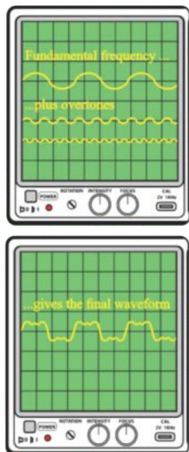
Fig: 11.6 Formation of a note on the oscilloscope
