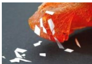
Fig: 14.3 The amber rubbed with silk attracts small pieces of paper
