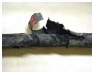
Fig: 15.23 Over heating of a cable
