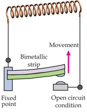
Fig 9.10 Bimetalic Thermostat
