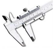
Fig 1.14 Vernier Calipers
