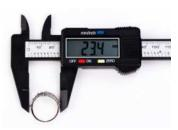
Fig 1.15 Digital vernier calipers
