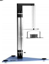
Fig 5.4 Extension in the spring depends upon the load.
