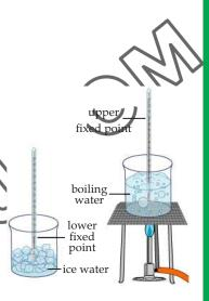
Fig 9.4 Heating ice experiment
