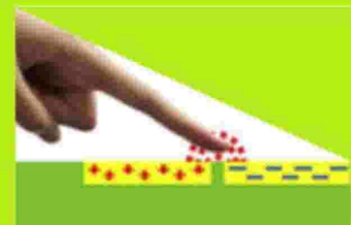
Capacitor also used as sensor
